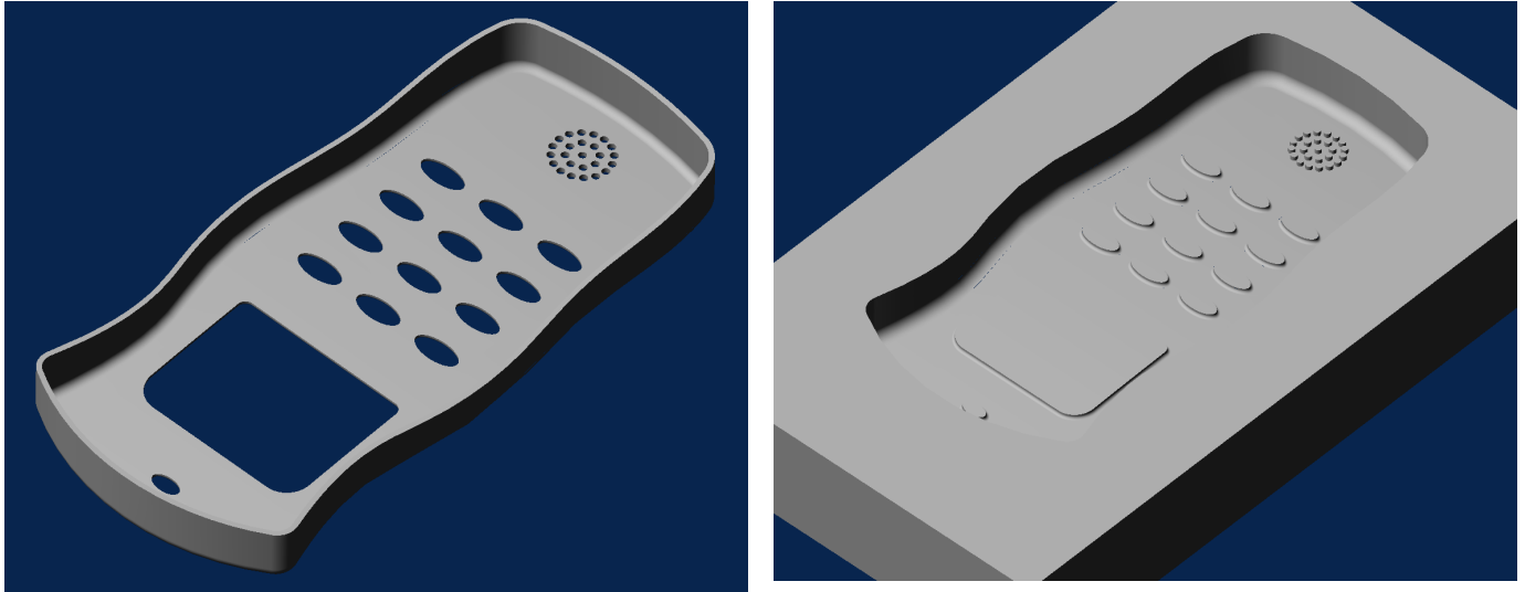
Figure 3 – The first two images above show a phone part and the mold cavity created from it. After more buttons were added to the part the cavity was automatically updated due to the new associative Booleans in Alibre Design 8.0 (image below).
